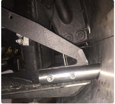
This conversion is for changing the "angle-iron" type Over-riders to a "tube" type that is suitable for mounting with a Sports Valance.
