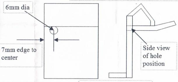
Drill 6mm dia hole.....7mm from edge of bottom bonnet catch and level with underside of lip.
